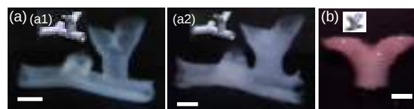
Fig. 11 Representative images of structures printed with drop-on-demand (DOD) approaches. (a) Inkjet-printed bifurcated structures, with (a1) alginate-only ink, allowing for higher geometric fidelity, and (a2) cell-laden inks. Scale bars: 3 mm. Reproduced from [181], with permission from Wiley Periodicals, Inc. (b) Y-shaped cell-laden alginate tubes printed using LIFT. Scale bar: 5 mm. Reproduced from [156], with permission from IOP Publishing Ltd.
