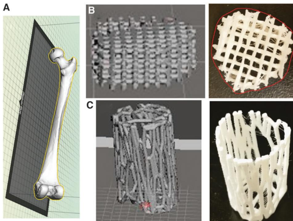
FIG. 3. (A) Cartesian data for a human femur were placed into the MakerBot Desktop. (B) A slice from the diaphysis of the femur was taken and Lattice meshed in Meshmixer. On the right is the 3D printed model in PCL. (C) Longer slice from the diaphysis was Voronoi meshed in Meshmixer to create a hollow cage-like representation of the outside of the femur. On the right is the 3D printed PCL model. Color images available online at [www.liebertpub.com/3dp](http://www.liebertpub.com/3dp)
