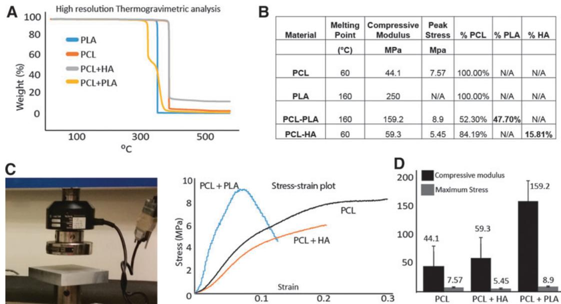
FIG. 2. (A) High-resolution TGA of polymer spools. (B) Results in tabular form showing the degradation points and percentages for each compound. (C) Compression testing apparatus to obtain mechanical properties of log-pile scaffolds. (D) Stress-strain plots and bar graphs of modulus and maximum stresses for each polymer spool. TGA, thermogravimetric analysis. Color images available online at [www.liebertpub.com/3dp](http://www.liebertpub.com/3dp)
