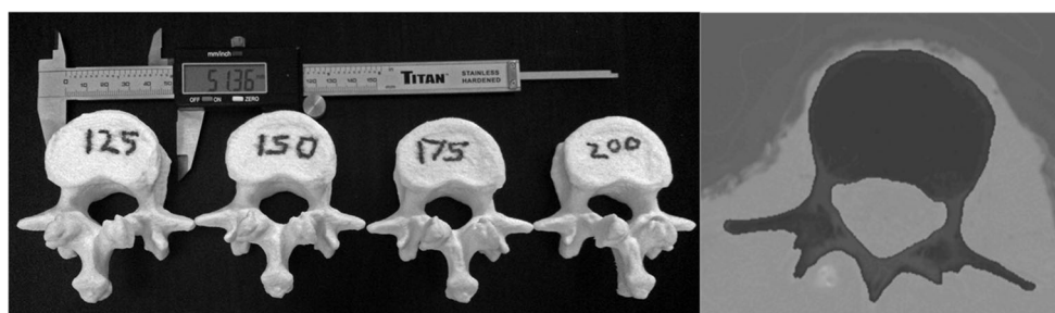
Fig. 2 Three-dimensional printed models segmented using varying lower threshold values for the semi-automated segmentation algorithm. The image on the right shows a typical CT slice through the vertebra with the shaded area representing the segmented bone
